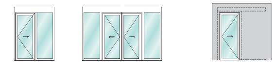
Janisol 2 EI30 fire-resistant sliding doors with "Break-In" emergency exit function (selection)
