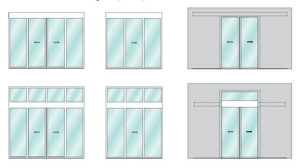
Janisol 2 EI30 fire-resistant sliding doors with "Break-Out" emergency exit function (selection)
